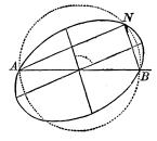
Through the point N, in which this arc intersects the ellipse, draw the supplementary chords AN, BN. Through the centre, draw two diameters respectively parallel to these chords, and they will be conjugate diameters, and make with each other the given angle.
